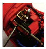
Replace the terminal of the new carbon brush
